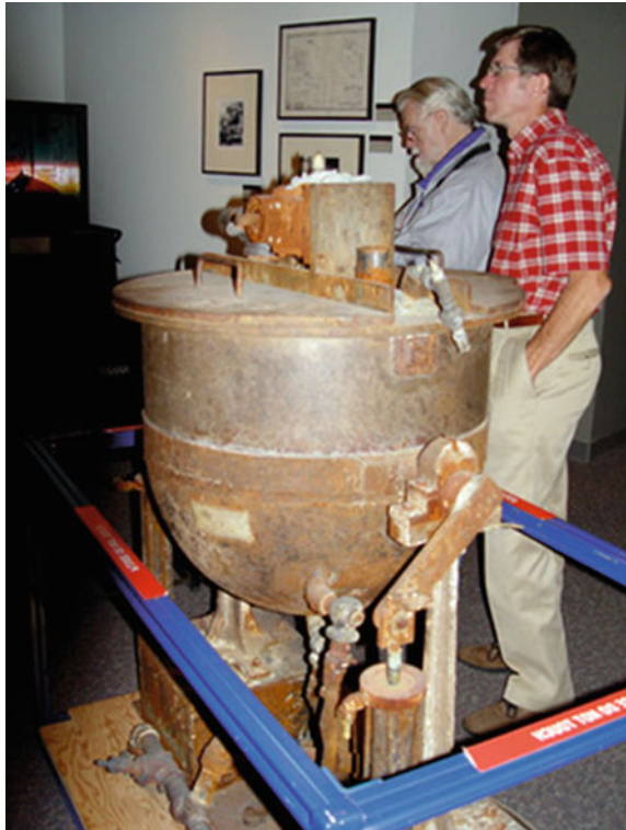
Fig. 7.22 An original implosion-lens casting machine on display at National Museum of Nuclear Science and History in Albuquerque, NM. Photo by author
