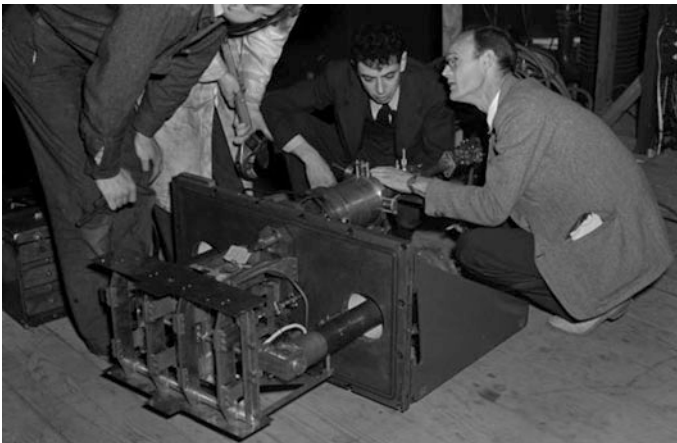
Fig. 5.16 Frank Oppenheimer (dark hair, center) and Robert Thornton (right) examine a 4-source Alpha-calutron ion emitter. Source http://commons.wikimedia.org/wiki/File:Calutron_emitter.jpg
